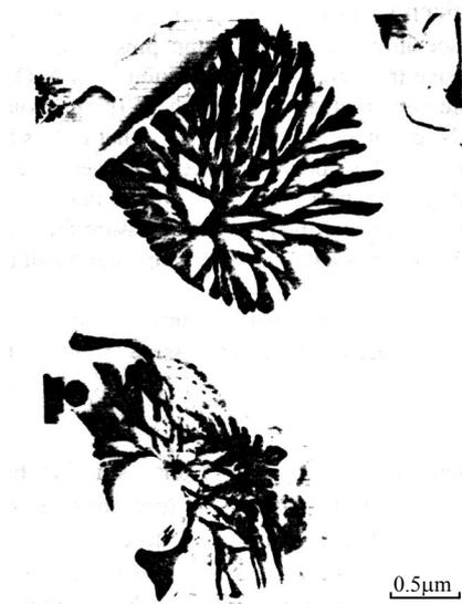
Fig.12 TEM bright field images of the interdentritic MC carbide in. well-developed, highly radially branching colony produced at cooling rate of  $1.4 \times 10^5$  °C/s (carbon Extraction replica)
